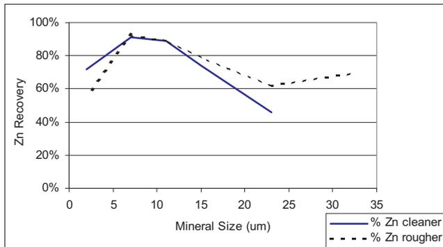
FIG 4 - Zinc recovery by size, cleaner and rougher circuit for tailings retreatment plant survey in 2007.
